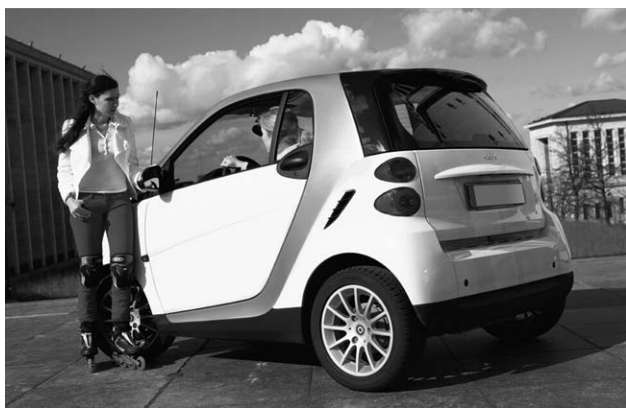
Figure 9. Smart Fortwo, a passenger car with in-color body panels molded from a composite based on a high-impact PP copolymer. Reprinted with permission from Borealis Co (copyright Borealis AG, 2008).
